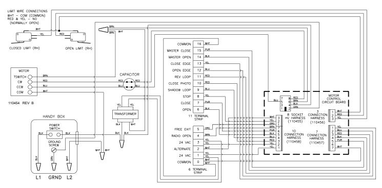
Figure 12: Schematic & Wiring Diagram
